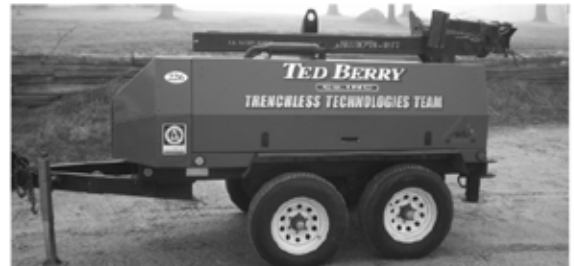
12 Ton Constant Tension Winch with 8" pneumatic hammer. For bursting municipal sewer lines made of VCP, CP, AC ect. Our HG12 Uses Patented Manhole exit.
